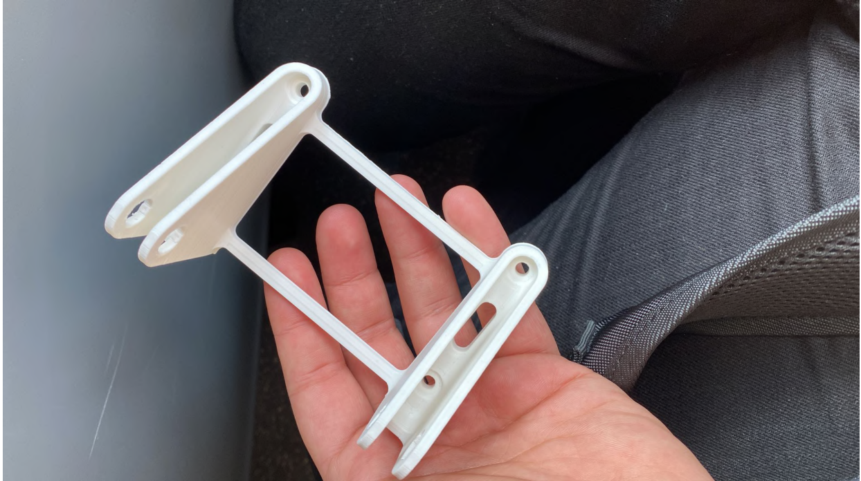
Figure 20: 3D-printed prototype of the wall bracket
